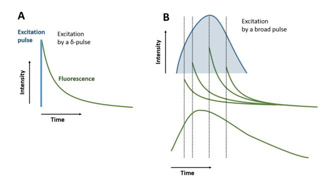
In practice, the excitation pulse width, the temporal dispersion of the fluorescence light in the instrument, and the detector contribute to the temporal response of the instrument, which has to be considered when analysing fluorescence intensity decays.
